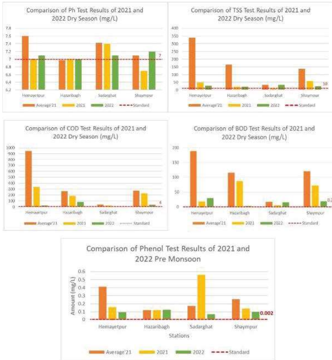
Figure 30: Comparison of pH, TSS, BOD, COD and phenol for the pre-monsoon season between the years 2021 and 2022
